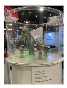
The Stäubli TX2 90 HE 6-axis robot demonstrates wash-down operations and waterjet cutting with two different protein products.
